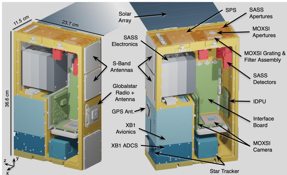
*Fig. 11. CubIXSS 6U spacecraft layout. Solar panels & instruments are Sun-pointed. Second solar array, top structural panel, and MOXSI metering structure are suppressed. [CLICK TO ENLARGE]*
