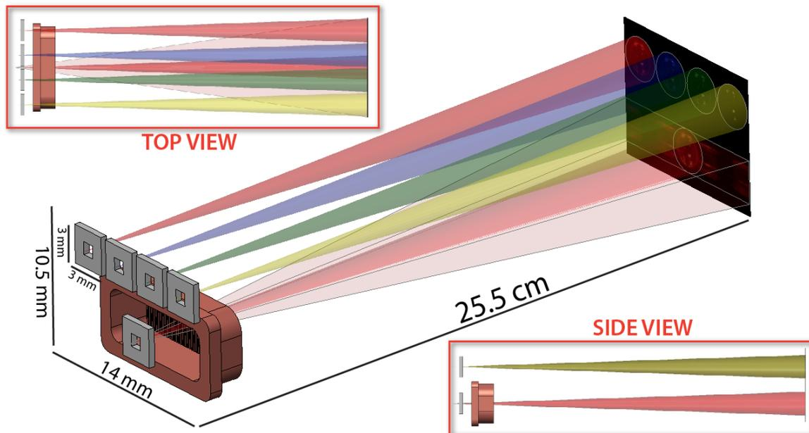
Fig. 8. MOXSI optical schematic. Four pinhole apertures provide filtergram images on the top half of the detector. Light from the bottom pinhole passes through the transmission grating to yield a spectrally dispersed image on the bottom half. (See also Fig. 7, above.) [CLICK TO ENLARGE]
