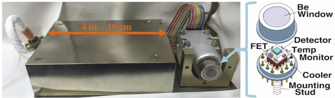
*Fig. 10. The X123 detector head is a sealed vacuum vessel including thermo-electric cooler (TEC) & beryllium window, with integrated preamp. The compact electronics include a complete multi-channel spectral analyzer and high- and low-voltage power supplies. The X123-FastSDD and -CdTe are identical in form, fit, and interface. [CLICK TO ENLARGE]*
