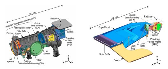
LEFT: Narrow Field Imager (NFI) is an externally-occulted compact-design coronagraph from NRL, with FOV similar to SOHO/LASCO-C3 (1.25° - 8° from Sun center). RIGHT: Wide Field Imager (WFI; 3x) is based on the STEREO/HI instruments and analogous to NFI in linear geometry, with a 40° wide truncated-square FOV centered 25° from the Sun.
