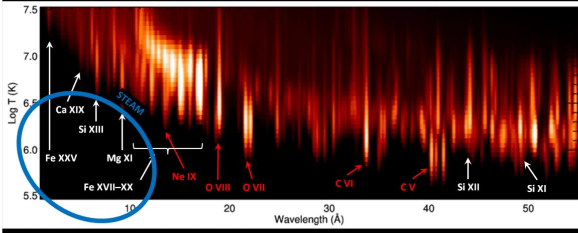
Figure 4: Above shows intensities of spectral line emission from various elements based on temperature (in Kelvin) and wavelength. Circled are the signatures STEAM will be focusing on based on our spectrometer capabilities
