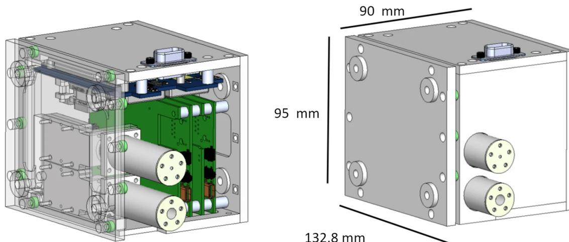
Figure 7: Above is a rendering of the STEAM instrument. Some exterior walls are not shown
